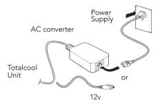
Connect ether the 12 volt or AC converter lead into the rear of the unit and then plug into your 12 volt or mains power.
