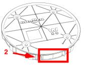
Fig. 5 Location of the battery pack.
