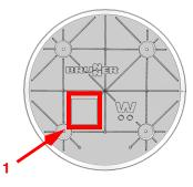
Fig. 7 Location of the type plate.
