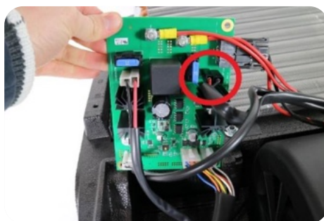
3) Disconnect the condenser fan connector from the bigger PCB
