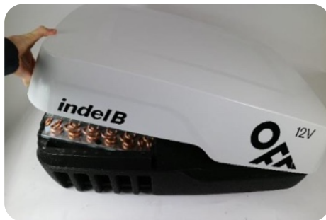
1) Unscrew the roof cover (5 screws)
