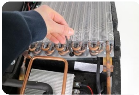
4) Unscrew the condenser (2 torx-screw)
