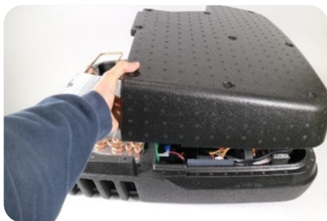
2) Remove the inner cover
