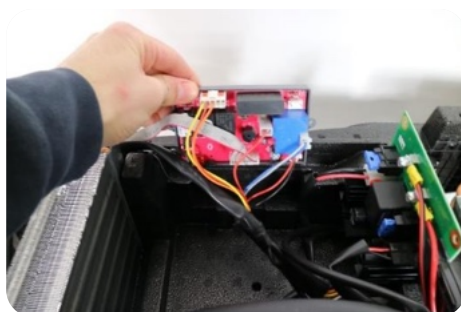
3) Slide out the main PCB
