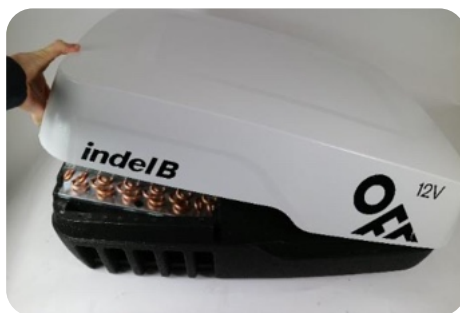
1) Unscrew the roof cover (5 screws)
