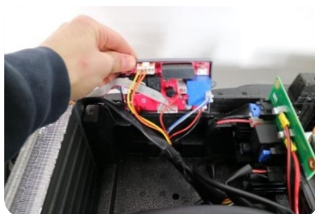
3) Slide out the main PCB
