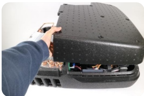
2) Remove the inner cover
