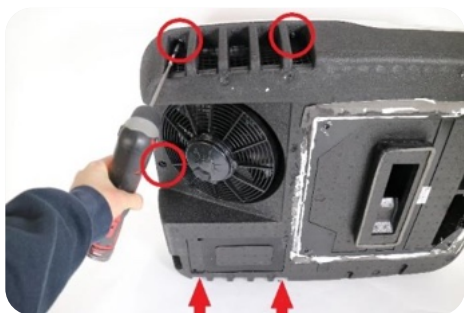
1) Unscrew the roof cover (5 screws)
