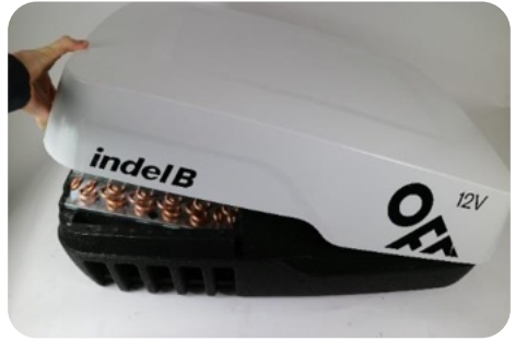
1) Unscrew the roof cover (5 screws)
