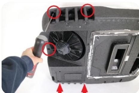
1) Unscrew the roof cover (5 screws)
