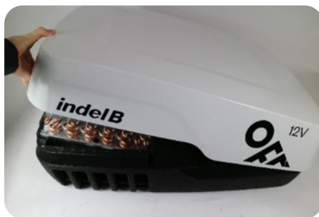
1) Unscrew the roof cover (5 screws)
