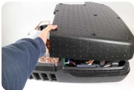
2) Remove the inner cover
