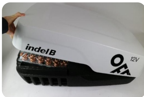
1) Unscrew the roof cover (5 screws)
