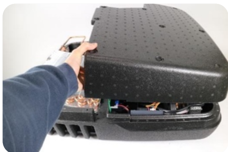
2) Remove the inner cover
