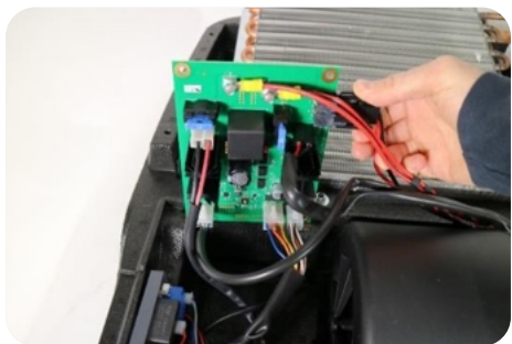
4) Disconnect all the connectors from the PCB
