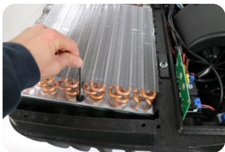
4) Unscrew the condenser (2 torx-screw)
