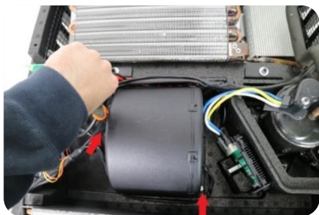
4) Unscrew the evaporator fan (2 screws-nut) and remove it
