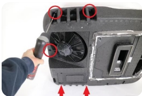
1) Unscrew the roof cover (5 screws)
