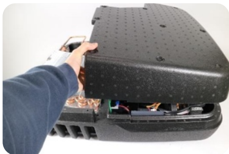
2) Remove the inner cover
