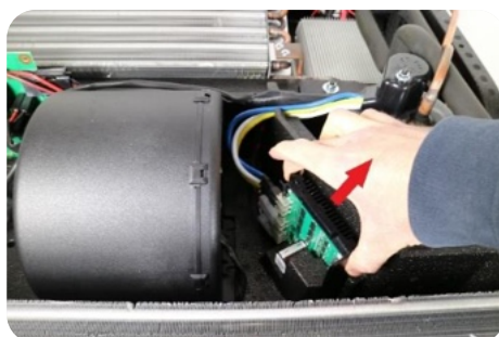
3) Slide out the main PCB
